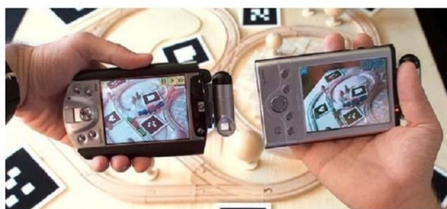
3.8 Gameplay demonstration of The Invisible Train . Individual player's PDAs show live video capture of the real, empty toy train platform overlaid with virtual trains and track switches. (The Handheld Augmented Reality Project, 2004)
